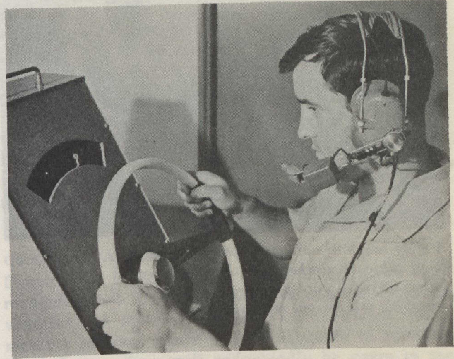
Subject tracks moving light on the stressalyzer as engineers and psychologists in the Control Systems Laboratory record his reaction and movement times.
