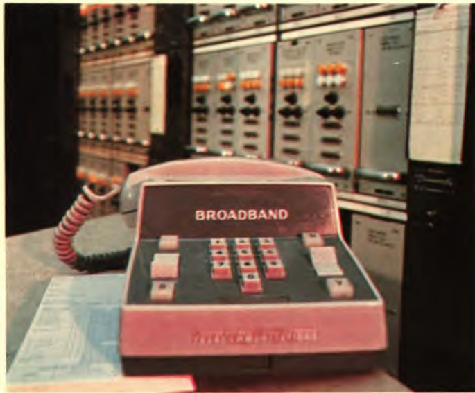
Canadian National/Canadian Pacific Telecommunications introduced its Broadband Exchange Service in 1967. The broadband computer communications network can send signals at high-speed over a wider portion of the electromagnetic spectrum than the telephone network.
