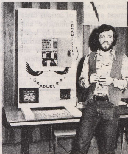
In the event of a power failure, the "gradulec" restores power gradually.
