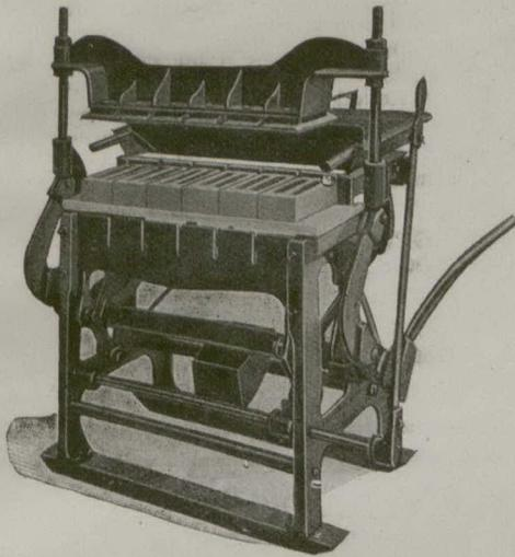
YOU can use fine gravel and crushed stone with this brick machine as it polishes the face of the brick, and therefore brings the cement to the face of the brick, thus assuring a much stronger brick in the face.
