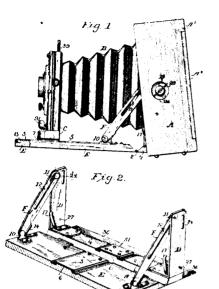
this latter is collapsed, supports inside of said box on which said box is angularly adjustable, and a camera bed having a hinge con-
