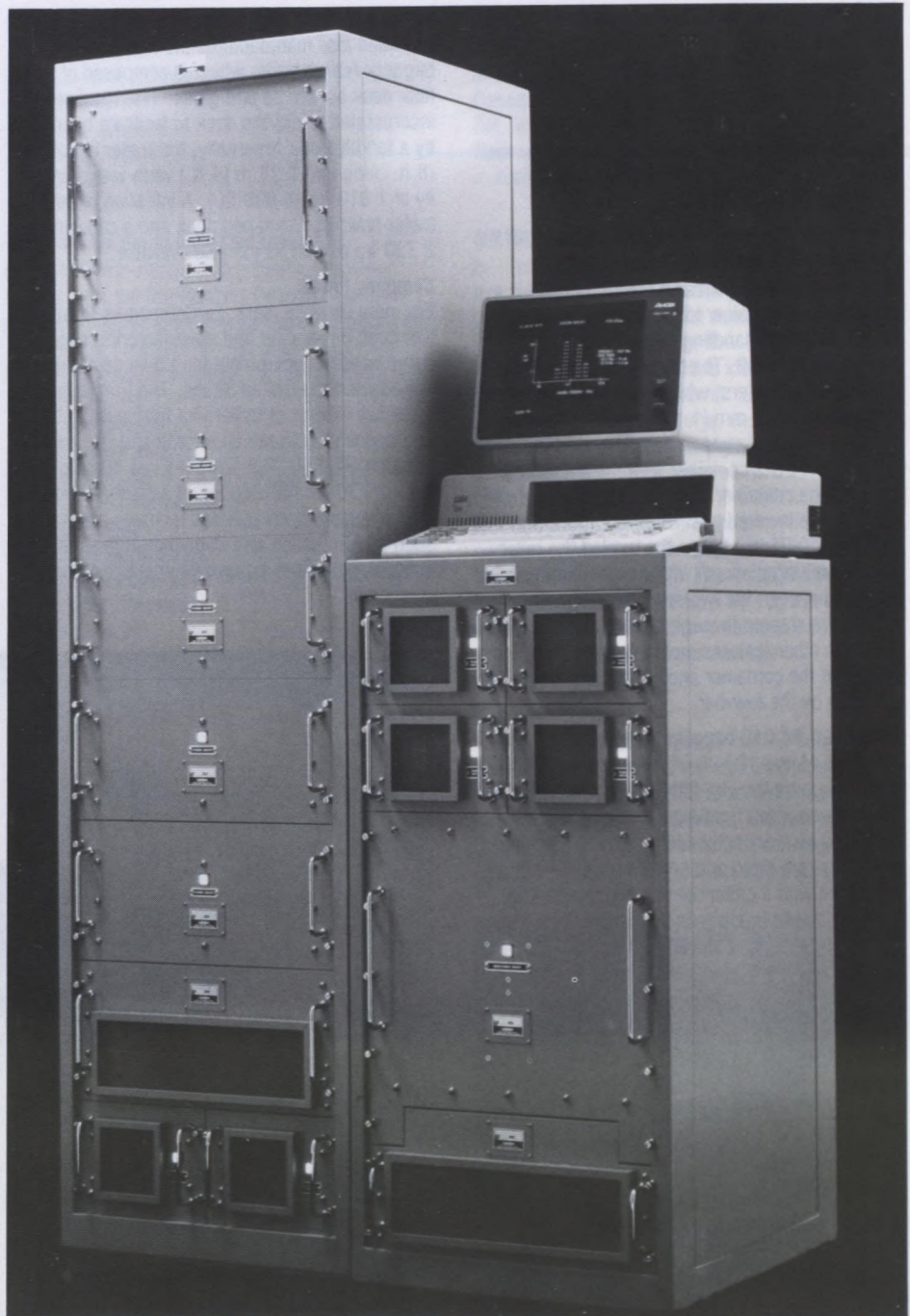
Tactical air navigation (TACAN) system
