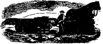
The thrashing machine represented in the above engraving is our vibrating machine. It has a run of a inches long with teeth in steel guaranteed so that they can bend without breaking as the norway. The from work that support the drills is all in wrought from which is very advantageous and economical as any blacksmith can make it, so that all long delays are avoided.
