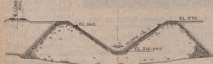
CROSS-SECTION AT STA. 335+00
