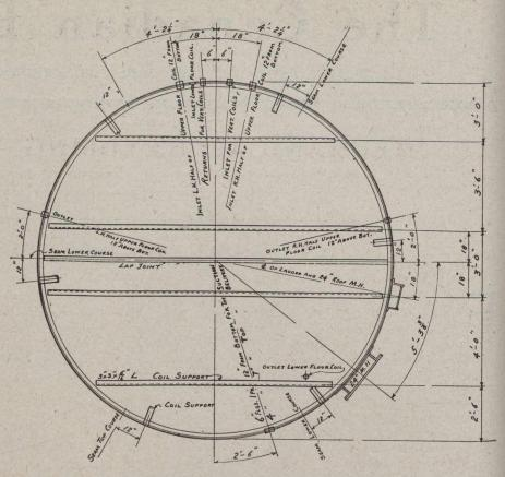
Sectional Plan of Tank Showing Location of Inlets and Outlets of Coils.
