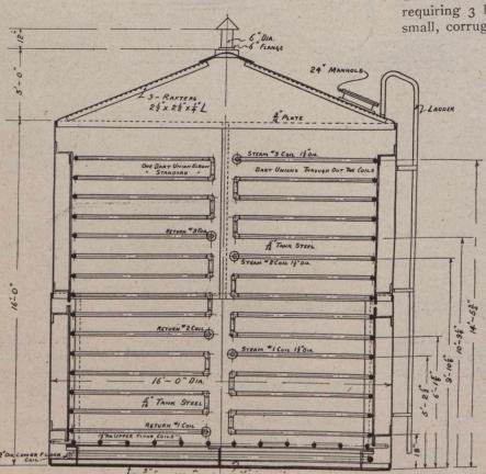
Sectional Elevation Showing Arrangement of Coils.
