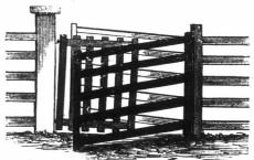
The gate swings in a V-shaped enclosure, or in two sides of a triangle; having top hinge the longest and the post plum; the gate, at rest, always hangs in the centre, and, rightly constructed, will always leave a passage way of two feet. Cattle cannot get through it. It is always shut and always open.
