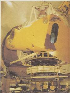
The eye of the telescope, its 3.66 m primary mirror, looks up from the circular support "cell" below the yellow beams. Whether used horizontally or at different angles, the mirror lies on a bed of pressurized air pads which keeps it from distorting under its own weight. The same Canadian-designed system was used in Victoria to cushion the mirror during the grinding and polishing operations. (Photo: W.J. Cherwinski)
