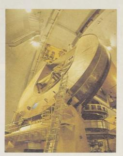
The 77 t horseshoe, at the so-called "north end" of the telescope, is supported by several brass-covered hydrostatic pads. When it rotates, the horseshoe rides smoothly on a thin film of oil, transmitting little vibration to the mirror. On most other telescopes, the gear drive for this kind of motion is located at the opposite end. The more elaborate CFHT system allows more accurate movement. (Photo: W.J. Cherwinski)
