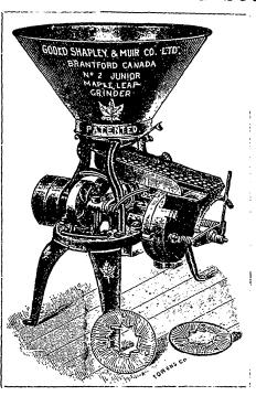
It is supplied with two sets of Grinding Burrs, goone for coarse grain and general purposes, and the other for hard grain and fine work.
