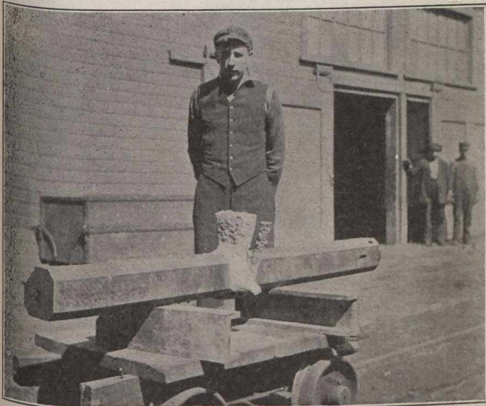
Fig. 1.—Cast iron boring bar of vertical boring mill.
