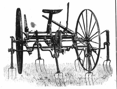
Is fitted with strong wheels, which have a double line of spokes like a bigycle.
