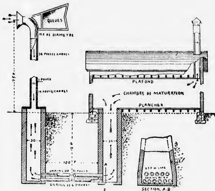
**DIAGRAMME MONTRANT LA DISPOSITION DES DRAINS DE VENTILATION.**
