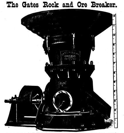
THE HIGHEST TYPE OF ROCK BREAKING MACHINERY! The Gates Gyratory Breaker is used on every Continent, having been
