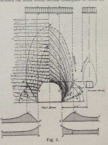
thrust of both the main and pioneer bores, in addition to the overlying weight, and crushing could then take place in a manner similar to that observed in the Simplon tunnel.
