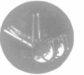
NO clogging troubles with these Discs. Notice how the space between boot and disc gradually widens from bottom to top. This prevents mud or trash stopping the discs from revolving. Scrapers are fitted accurately to the
