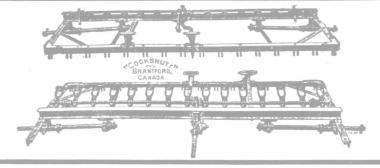
THIS frame carries the weight of the grain box. It is made of heavy high carbon angle steel, reinforced with malleable corners and steel corner braces.
