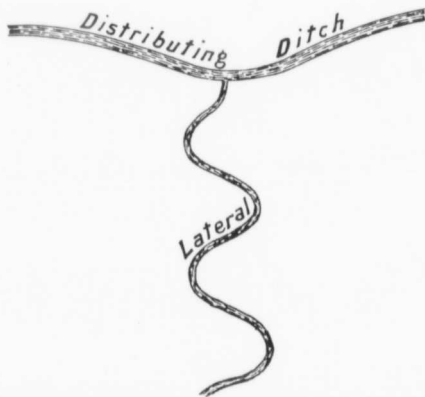
Fig. 17 - Ditch running down steep slope
