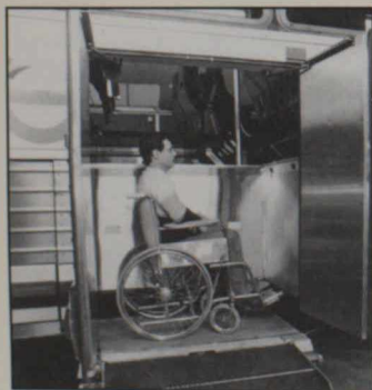
Computer-controlled bus lift undergoing trials with TerraTransport of Newfoundland.
