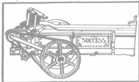
Built with more strength than will ever be tested in use, devised so it cannot clog. Gear that controls apron feed and regulates volume of spread, runs in an OIL BATH—so it stays in order and runs easy always.
