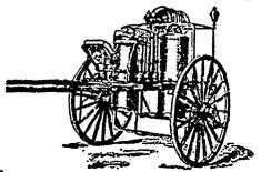
This machine is the most powerful fire fighter. It has two cyl'nders, 40 gallons capacity each. The combination of chemicals will not freeze, renders material with which it comes in contact non-inflammable, and will not corrode when not in use. For full particulars, write to the Head Office of the Company at Kingston.
