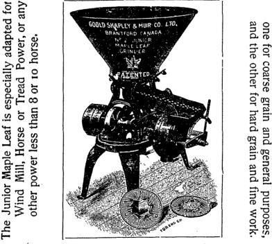
The Patent Ball-Bearing takes the heavy back pressure of the burs when at work, and greatly lessens the friction. In consequence the Grinder will do more with a given power than any other.
