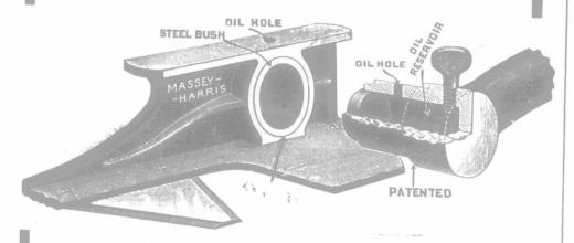
The oil is drawn up by suction through the oil hole by the natural action of the Pitman.
