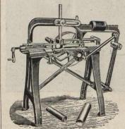
Cuts Bars 6 x 6, either round or Cuts Bars 6 x 6, either round or square. It requires no attention after work is put in vise, and stops automatically when piece is cut off. We would especially call your attention to the IMPROVED ARM, which keeps the saw perfectly in line at all times.
