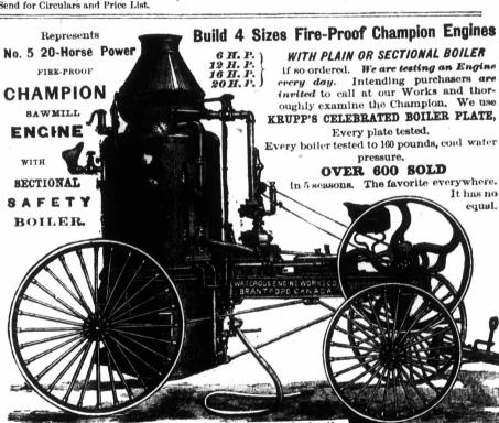
The sectional safety boiler is manufactured expressly for the "North West" trade. This boiler is so arranged that it is readily taken apart in sections enabling purchasers to clean thoroughly every part of it and prevent burning out. We know from experience this is absolutely necessary with the alkaline waters of the great Western prairies. Largely used by the Pacific Railway Company and all the large Colo-
