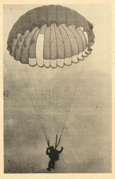
the student is ready to make his or her first "static-line" descent. A static-line is a device which ensures proper opening of the parachute, regardless of the actions of the jumper.
