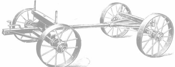
A cheap wagon for the farm, made with wide-tire iron wheels, and built low to facilitate loading and unloading. Carries a heavy load, runs easy, and won't cut into the ground.
