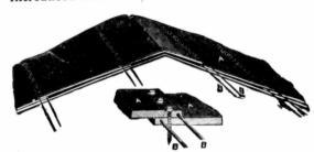
A shows method of laying Red Star Brand Wire Edged Ready Roofing, with 2-inch laps secured by nailing two inches apart. BB shows wires running through the edges of the roofing, giving it great strength at the joints or laps—a very desirable feature, especially in localities where high winds prevail.
