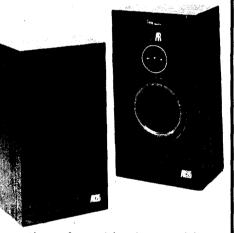
The AR25 includes AR innovations found in the world-famous AR9. THe AR25 is a two-way system with a vertical driver array to guarantee a crisp stereo image. In addition, the liquid-cooled tweeter uses magnetic fluid to dissipate voice coil heat, permitting greater power handling in the speaker. A two-position crossover switch adjusts the high-range level.
