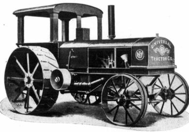
25 H. P. is the latest in double opposed cylinder all gas power, and is untype, 7½ inch bore by 8 surpassed as an economic inch stroke. Speed 500 ical, durable and reliable revolutions, 40 horse gas engine.
