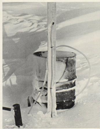
of a U-shaped piece of plastic tubing filled with diesel fuel. Its ends were raised and fitted with calibrated glass tubing. The difference between fuel level readings taken at both ends indicates platform tilting behavior.
