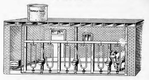
This cut illustrates the method of using our PATENT STABLE FIXTURES, and we ask that it be carefully examined. Only a light wooden frame is necessary to support the Stanchions. No partitions or wooden mangers are necessary, consequently every part of the stable is light and airy with no dark corners to accumulate dirt.
