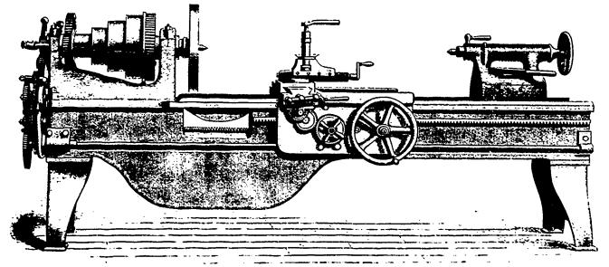
This Cut represents our NEW GAP LATHE, with inverted V Shears, extra heavy, to which we call special attention. These Lathes are built in lots of not less than 12, thereby ensuring accuracy of detail, and parts Interchangeable.
