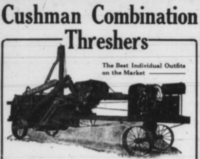
The Famous Light-weight Cushman Engines, mounted on same truck with Separator:
