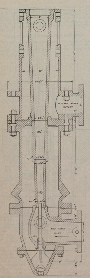
FIG. 5—SANDWASHER APPLIED TO PRESSURE FILTERS AT ROCKLAND, ONT.
