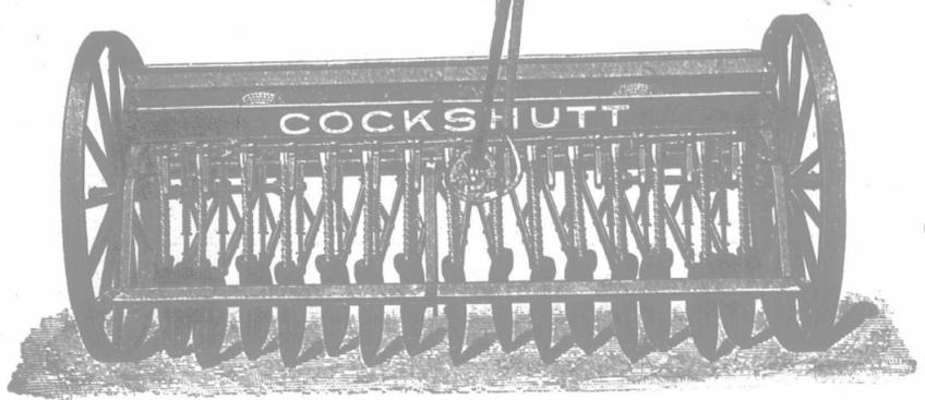
**T**HE great feature of this Cockshutt Disc Drill is its very light draft and even seeding at even depth. The light draft is obtained from self-oiling dust-proof disc bearings and perfect fitting parts. The even seeding is maintained by a protected feed device, not subject to jarring from the wheel action. Seeding at even depth is attained by a steel I-beam frame, which holds up both the discs and grain-box, no matter how rough the usage or wear given the drill.
