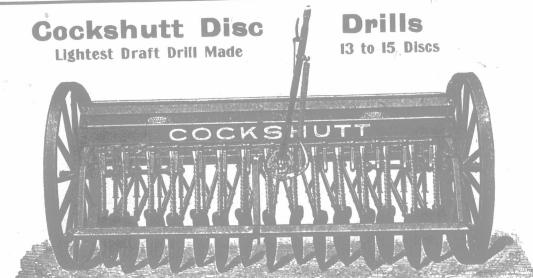
THE great feature of this Cockshutt Disc Drill is its very light draft and even seeding at even depth. The light draft is obtained from self-oiling dust-proof disc bearings and perfect fitting parts. The even seeding is maintained by a protected feed device, not subject to jarring from the wheel action. Seeding at even depth is attained by a steel I-beam frame, which holds up both the discs and grain-box, no matter how rough the usage or wear given the drill.
