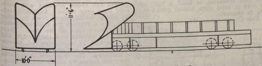
Fig. 4. Snow Plough, attached to Ballast Car.
