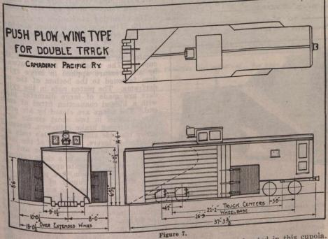
down to within 8½ in. of the rail, in order der to within 8½ in. of the ran, the front truck. The bottom portion is hinged
