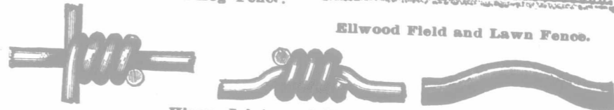
Hinge Joints and Tension Curves.
