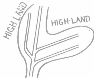
Fig. 4.—Drains adapted to suit the land.
