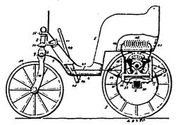
standards supported upon said axle, lift-screws engaging the same, learing-boxes carried by said lift-screws and engaging the motor-shaft near its opposite ends, arms mounted rigidly upon said lift-screws, and means to operate the same so that the motor-shaft will be raised or lowered, substantially as set forth.
