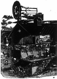
Geared Windmills, for driving Machinery, Pumping Water, &c., from 1 to 40 horse-power. . 247-a
