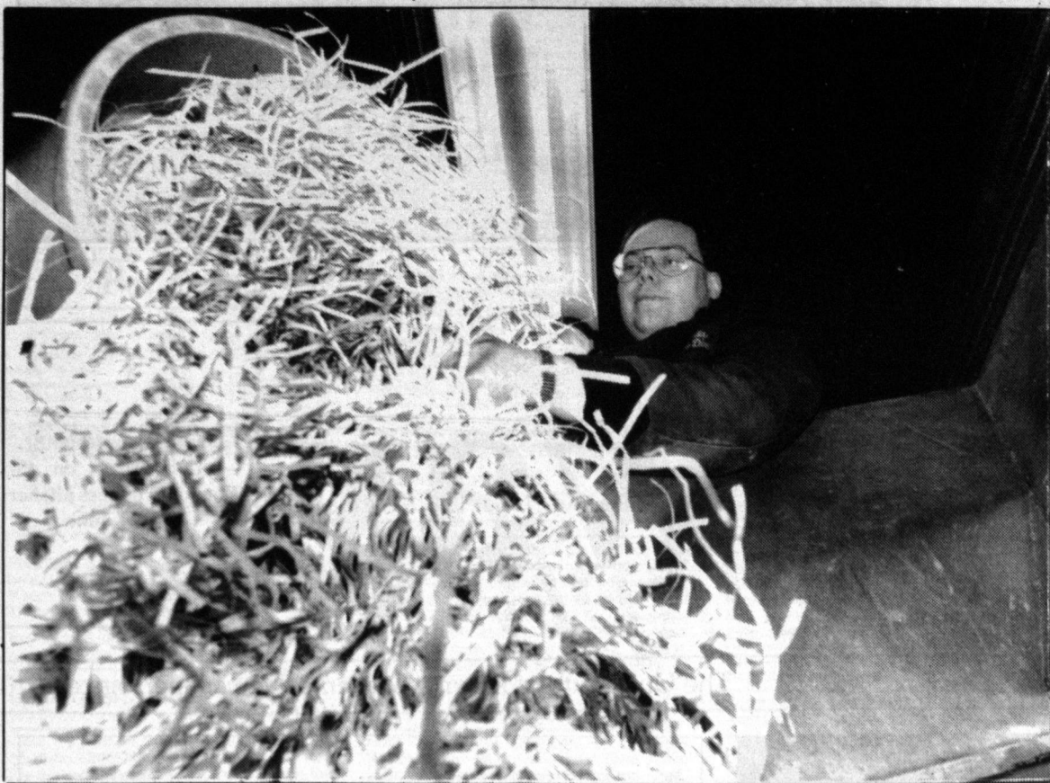
Mark McQuitty of building services loads some shredded confidential documents into a bailer. The machine bails the paper into 600 lb bundles that are then sold to a recycling firm.
