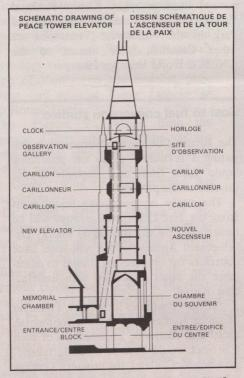
The renovations will make it easier for the 5,000 visitors wanting to travel to the top of the 76.5-metre (255-foot) tower each year. Safety glass is being installed to replace the wire barrier on the observation level and will provide a better view to visitors. Special viewing windows will be cut in the stone at a low levels for children and people in wheelchairs.
