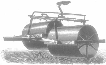
The bearings are the only wearing parts, and are guaranteed to last from Ten to Fifteen Years, and can be replaced at a nominal cost. It rolls all the ground, no matter how rough. There is no axle shaft, no strain, and consequently no wear. It is easily oiled between the drums.
