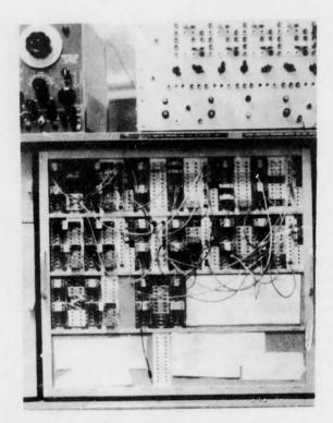
Electrical Engineering Above is an analogue transistorized computer. It is part of a set up for simulating the response of automobile suspension, aircraft control systems, etcetera.
