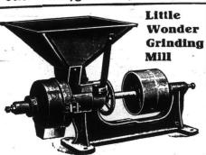
Especially adapted for gasoline engines. Most successful little grinder in the world. Made of iron and steel and has few wearing parts. It is not liable to get out of order. Will run empty without in jury to burs. Grinds all kinds of grain. Grind from 5 to 15 bushels per hour if run from 600 to 1,200 revolutions per minute. Requires 1 to 3 b.p. to operate. Burs are 5 in.. drive pully 6 in. weight 90 lbs. Price, complete with two sets of burs. \$10.50,
