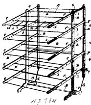
provided with openings 2, and pivoted through said openings to said standards, connecting bar E, pivoted directly to the upper and lower of said arms, and toggle F, pivotally connecting said bar E, and the intermediate arms C, substantially as shown and for the purpose described.
